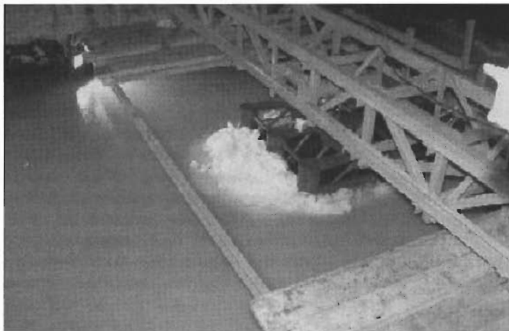
Fig. 5 Forming ice rubble accumulations in front of IRP-1 model when pushing level ice sheet
